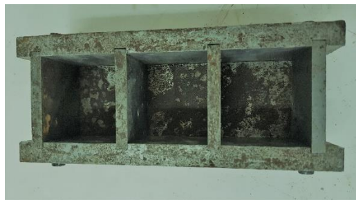
Figure 2 : Cubic moulds (50 mm x 50 mm x 50 mm) for density and compressive test according to ASTM C473-12.
